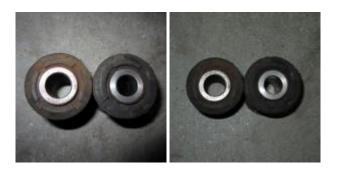
An important thing to note is the rear inner bushings will have a larger inner diameter on the metal collar. This is for the eccentric bolts that adjust toe – all of the rest of the bushings should have the same size for the inner metal collar. Make sure you put them in the correct location!
