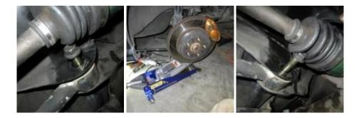
On some of the nuts you might need to get another combination wrench on the other side so you can get the nut out without spinning the bolt. You may also need to jack up the hub to get some clearance for some of the bolts, otherwise they will not clear the CV boot.
