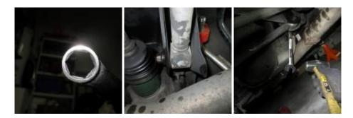
Start inboard near the center of the car. Take your 6 sided 17mm box wrench and PB Blaster, and start by removing all of the nuts holding the inner ends of the lateral links in. Beware that as soon as you remove the nut on the rear inner lateral links, your alignment (specifically your rear toe) WILL be buggared. Make sure you take note how the eccentric bolt and eccentric washer are installed since those are used to set your rear alignment.There's no going back now!
