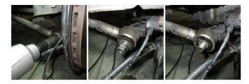
The outboard ones are a bit more of a pain in the ass. See that long bolt that goes through the hub? I'll bet you that yours is seized in the hub like mine, so that is why we removed the inboard bolts first. You should be able to get an impact on the nut on the hub – that nut gave me no problem. The nut side should be facing forward – since this bolt is so long, you need to get the impact gun on the nut side or else it's not going to do anything.
