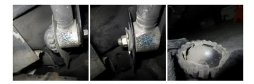
The forward inboard nuts have little covers on them that you need to twist off. Take the bolts out, let the lateral links hang loose. I've been told these plastic caps are to protect the fuel tank from being punctured when the car is involved in a collision.
