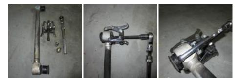
The soft aluminum used in the lateral links damages easily. For the ends with just the bushings in them, the jaw puller will work, just be careful. For the ends with the long bolt stuck and fused to the bushing, I made a trip to the local machine shop and opted to have the machinist press those bushings out. Those bushings come out on the press with no drama because there's no metal collar on them. Your long bolt is probably going to be fused to the metal sleeve on the collar.
