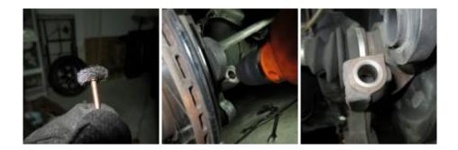
With the bushings out, get a wire wheel and a high speed corded drill and polish away the inside surfaces of your lateral links. They don't have to be perfect mirror shiny, but make sure to remove all the surface rust and old bushing material that may be stuck on them. Do the same for the hub where the long bolt goes through.
