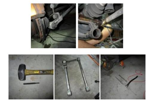
When you take the lateral links out, make sure you mark which one is forward, which one is rear, and which direction each one faces. They are not symmetrical.
