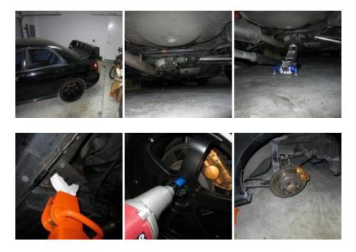
Jack up the rear of the car using a floor jack – I found the easiest way to jack up the rear of the car is to raise the car from the rear differential. A few pumps and the car is off the rear wheels. Put jackstands under the rear subframe mounts and remove the wheels. God help you if you need detailed instructions for this.
